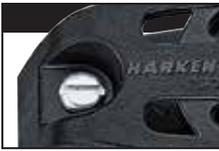
Using block as template, mark holes using a centerpunch. Remove block and drill holes using a  $1\frac{1}{64}$ " (4.2 mm) drill. Bevel top of deck holes using a small knife to allow sealant to mass. Through-bolt block using recommended stainless steel fasteners, washers and locknuts.
